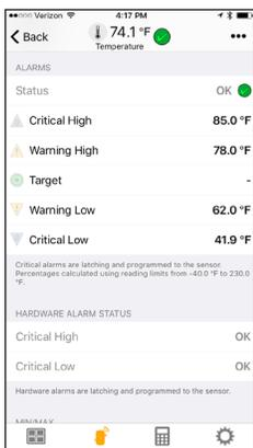
Define measurement thresholds to get notified of important changes. Critical thresholds are programmed to sensor firmware for exception monitoring between readings.
