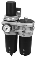
Filter / Regulator + Lubricator Combinations 5 micron element, 12 bar (174 psig) regulator + gauge and wall mounting bracket
